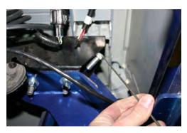
6. Fit bolt plate into chassis down through support gusset in Kaymar bar using M12 flat, spring and nut. **DO THESE BOLTS UP FIRST**.
